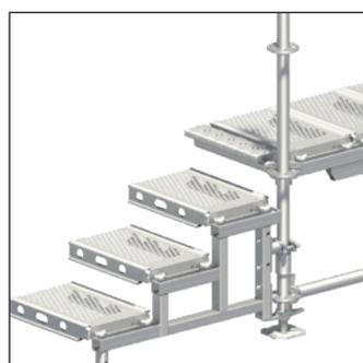
Adjustment to the ground, with access to the first scaffolding level, can be achieved with the Allround modular stair. The construction kit comprises: stringer for modular stair with 1, 2 and 3 steps, base collar for modular stair 0.26 m and O-ledger LW 0.90 m. 0.32 m-wide standard scaffolding decks in the selected length are installed as steps. The steps are fastened using lift-off preventers.
