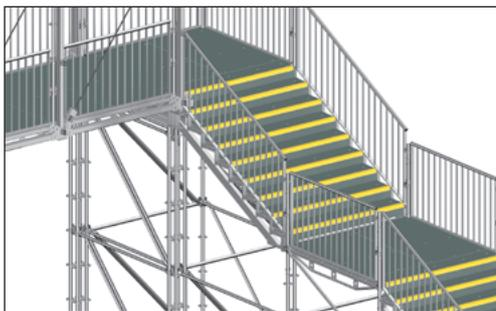
Sure footing with Layher step covers. With their non-slip surface using quartz sand, they ensure maximum safety on Layher stairs in rain, snow and ice conditions. The step covers are made from glass-fibre-reinforced plastic. They are permanently resistant to weather effects, easy to clean, electrically non-conductive and flame-retardant. They can be fitted quickly and are optimally matched to the Layher stair range.
