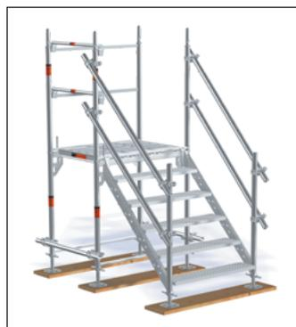
With the Layher modular stair, accesses can be constructed that always fit and match the system. Any intermediate dimension with a pitch of 20 cm can be achieved simply by fitting together the individual stairway parts. The top element is suspended in the U-section of either the assembly frame or the Allround ledger. At the bottom, the end section with scaffolding spindles is used for precise levelling.
