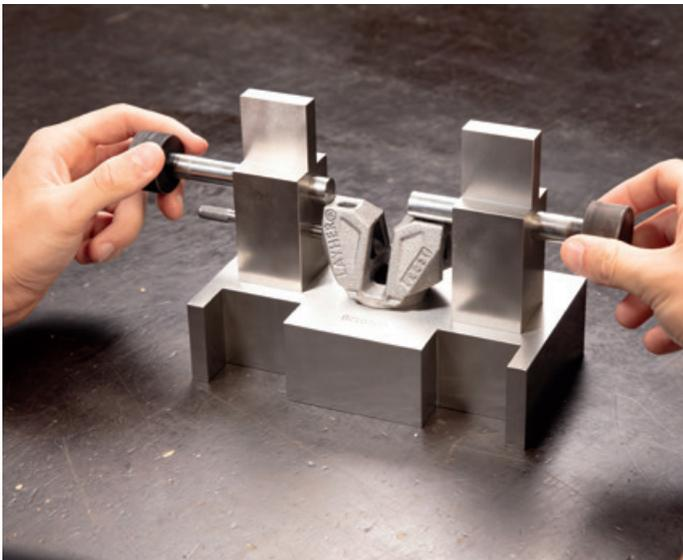
Dimensional and function test of the semi-finished parts
