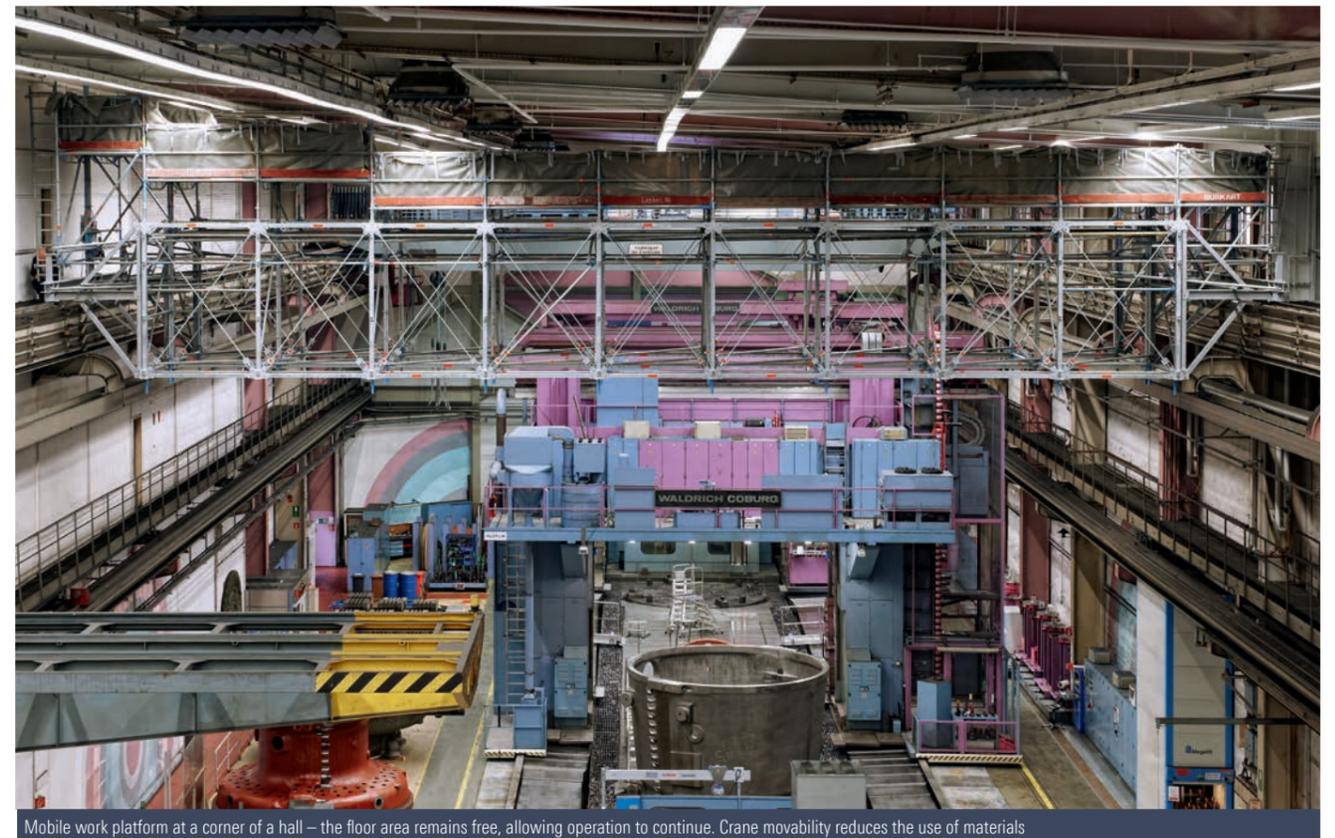
Mobile work platform at a corner of a hall – the floor area remains free, allowing operation to continue. Crane movability reduces the use of materials
