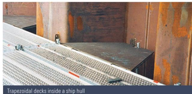
Trapezoidal decks inside a ship hull
