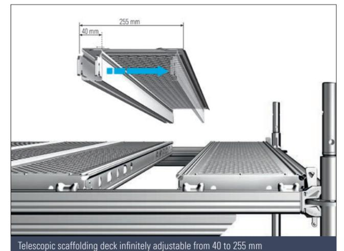
Telescopic scaffolding deck infinitely adjustable from 40 to 255 mm
