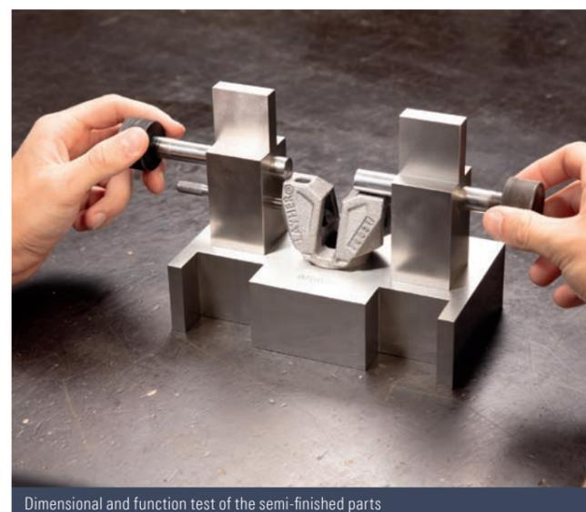
Dimensional and function test of the semi-finished parts
