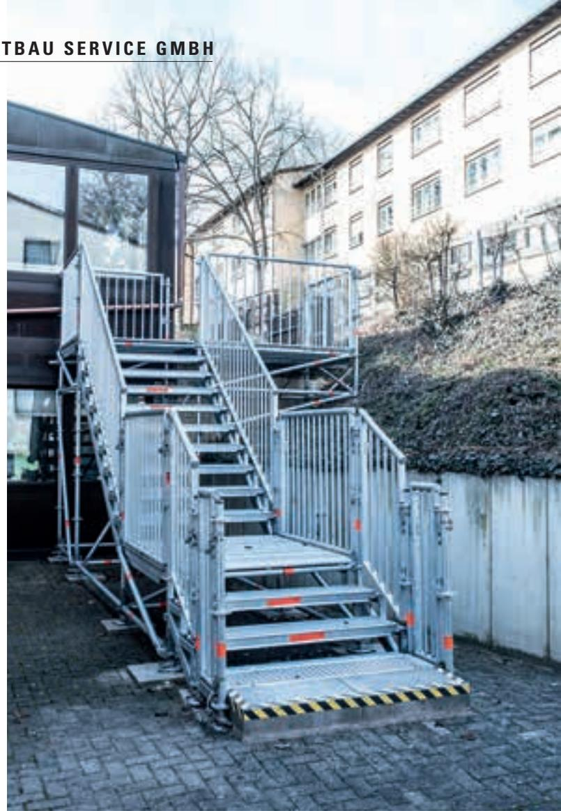
▶▶ With the proven Layher Allround Scaffolding, the stair structures can be adapted to specific building architecture, e.g. exit heights. The pitch dimensions and load bearing capacity of the Layher stairway tower 750 make it ideal for escape stairtowers. Unlike custom-made steel and wood fire escapes, the modular Layher Allround Scaffolding offers the benefits of fast and cost-effective assembly.
