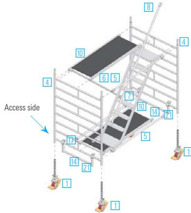
Insert the castors **1** into the ladder frames **4** and secure against falling out by fastening the wing screws on the spindle nuts.
