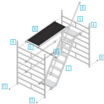
During assembly and dismantling, system decks or scaffold planks according to DIN 4420-3 (minimum: 28 x 4.5 x 220 cm long) must be used as auxiliary decks at maximum height intervals of 2.0 m. These auxiliary decks provide a safe footing for assembly and dismantling, are removed after the erection. Each platform must be completely boarded.
