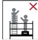
It is not permitted to increase the platform height by using ladders, boxes or other mechanisms.
