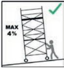
Movement is only permitted on sufficiently firm ground with a max. inclination of 4% (approx. 2.5°), in the longitudinal direction or perpendicular to this, and the speed must not exceed normal walking pace (4 km/h). All impacts must be avoided.
