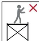
It is not permitted to stand and move around on unsecured levels/platforms of mobile working platforms.
