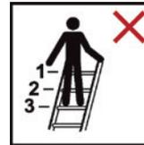
Do not use the top three steps/rungs of a simple ladder to stand on.
