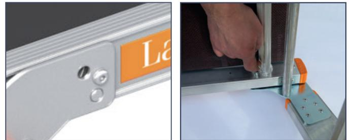
Before using the working platform, the two access ladder sections on the right side and left must be pushed completely outwards and locked in place, so that the working platform is stable. The working platform can then be used.
