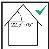
The ladder may only be used on roofs with inclinations from 22.5° to 75°.
