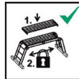
When using the ladder as a platform may only be recommended by the manufacturer. Platform elements are used. The Platform element must be before use be secured.
