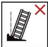
Do not use the ladder on an uneven or unstable surface.
