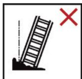
Do not use the ladder on an uneven or unstable surface.
