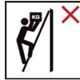
When using a ladder, do not carry equipment which is heavy and awkward.
