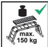
Observe the maximum load of the pedestal specified by the manufacturer in scaffold position.
