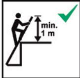
Ladders for access to greater heights must be extended at least 1 metre above the contact point and secured as necessary.
