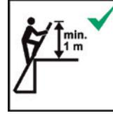
Ladders for access to greater heights must be extended at least 1 metre above the contact point and secured as necessary.
