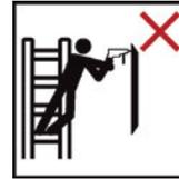
Avoid any work exerting a lateral load on the ladder, for example drilling sideways through solid materials.
