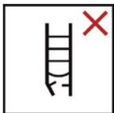
Check ladder upon delivery. Visually check the ladder for absence of damage and for safe use prior to every use. Do not use damaged ladders.
