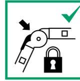
The locking bolts on the hinge plates need to be engaged on both sides and thus secured before use.
