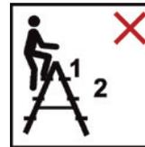
Do not use the top two steps/rungs of a double ladder to stand on without a platform and a holding device for the hand/knee.
