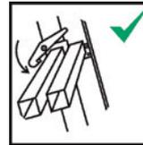
Locking devices must be fully activated before the ladder is used, if this is not done automatically.
