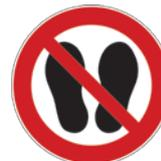
Horizontal surfaces resembling the platform of a double ladder but not designed for that purpose (e.g. plastic work tray) must be clearly identified on their surfaces, if necessitated by the design.
