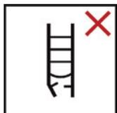
Check ladder upon delivery. Visually check the ladder for absence of damage and for safe use prior to every use. Do not use damaged ladders.
