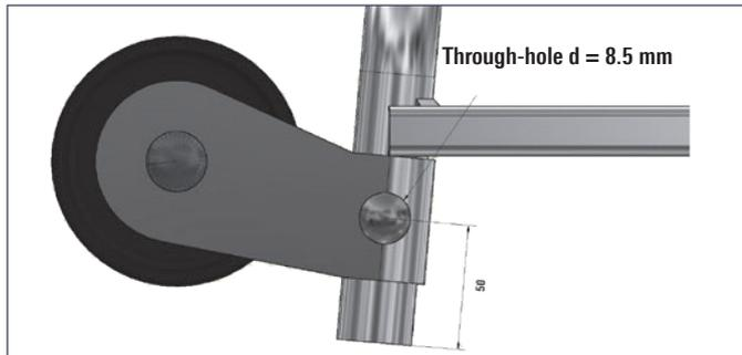
1. Drill a through-hole at the two rear marked ends of the machine tread.
