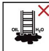
Do not set up the ladder on a fouled surface.
