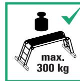
The maximum load of the platform must be observed.
